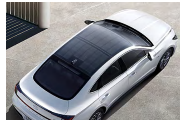
Solar Roof installed to an electric vehicle
